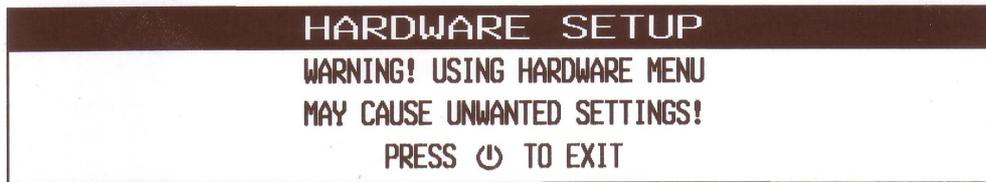
Then press FEED button, to enter Hardware menu. Device will prining current settings.
